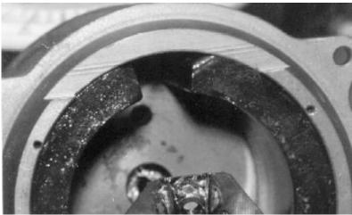
**Botview.jpg** The lower surface is shown along with the detector coil itself. A short stub on the input of the amplifier allows the coil to be shorted in order to evaluate the amplifier noise level.
