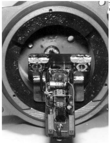
**Topview.jpg** This shows the component side of the detector electronics module and the mechanical supports. The magnets and open end of the detector housing are visible.
