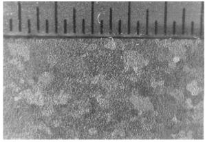
**Coremat1.jpg** This was originally an unenhanced 256 level gray scale image produced from a photographic closeup of the detector core material. Note the size and contrast of the crystal grain structure. The scale visible along one edge of t he material is calibrated in 1/16ths of an inch.
