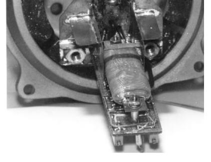
The circuitry is constructed on "pad per hole" protoboard, with all component leads bent flush along the board, and then soldered to the copper pads. This technique can produce a finished board that is more rigid than a printed circuit board. The finished amplifier board is then soldered to copper strips that form the mounting supports. The detector coil is attached directly to the amplifier by short spacers. The Barkhausen effect core material itself is grounded.
