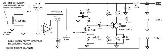
SCHMT1BC.GIF Schematic of the Beta Prototype detector
